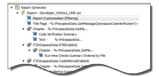
**b** Select the **Report Customization (Filtering)** component. On the right pane, you can set the properties of this component. By default, the properties are set such that all results are included in the report.
