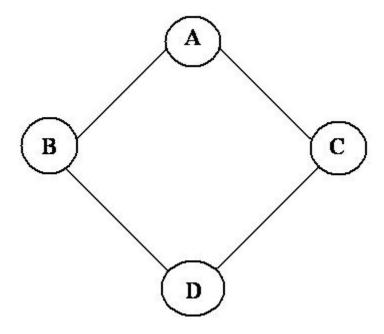
B and C classes virtually inherit the A class
