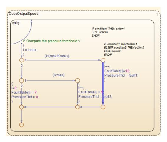
You can avoid the **Out of bounds array index** in several ways. One way is to constrain the input variable index using a Saturation block before the Stateflow chart.
