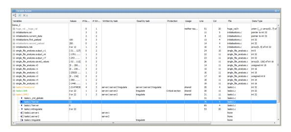
The function, Tserver, in the file, tasks1.c, performs two write operations on SHR2. This is indicated in the **Variable Access** pane by the two instances of
