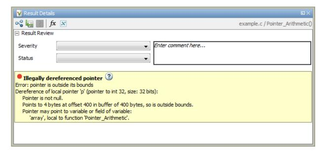
For details on the information available for each check type, see "Types of Run-Time Checks" on page 8-47.
