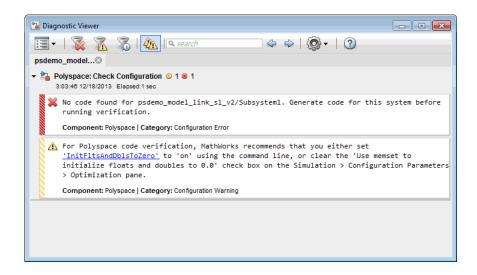
If you alter your model settings, rebuild the model to generate fresh code. If the generated code version does not match your model version, the software produces warnings when you run the analysis.
