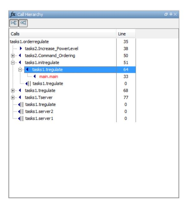
Depending on the name, the corresponding line number in the **Call Hierarchy** pane refers to a different line in the source code:
