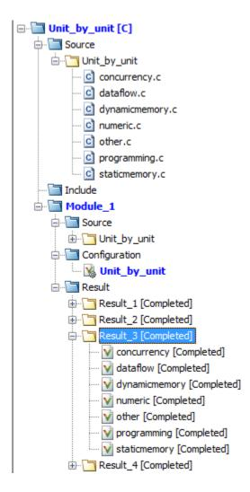
After a source file is verified, to open the results, double-click the corresponding result file under the **Result** node. Alternatively, after all source files are verified, you can see a summary of results for all files and begin reviewing from files with more severe issues.
